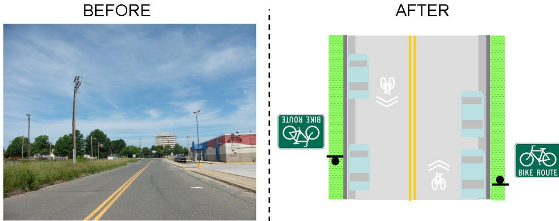
Figure 20: Before and After Signage/Striping Improvements for Marshall Ave.
