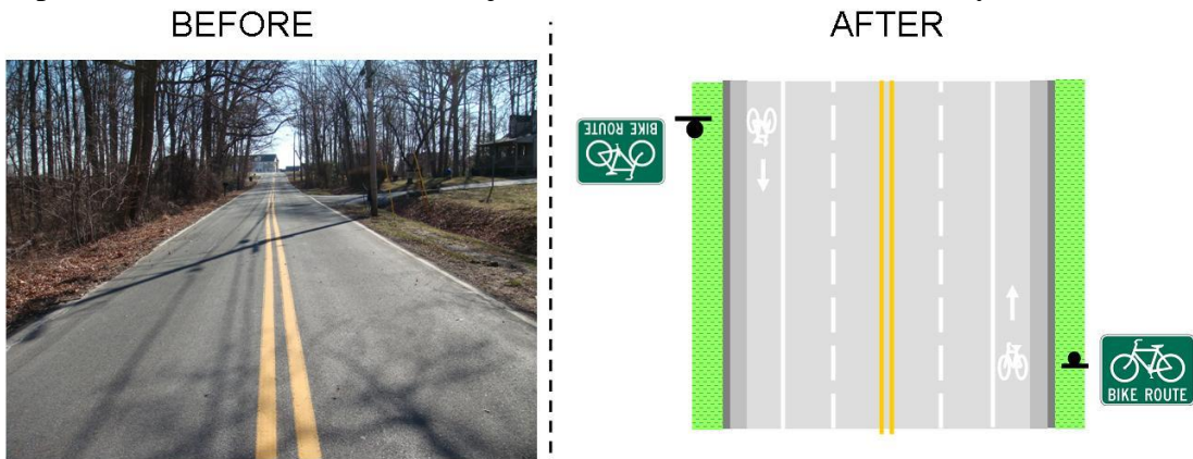
Figure 11: Before and After Signage/Striping Improvements for Cherry Lane.
