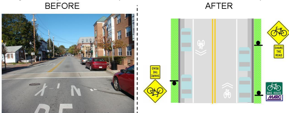
Figure 19: Before and After Signage/Striping Improvements for Main St.
