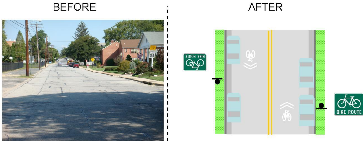
Figure 10: Before and After Signage/Striping Improvements for 8th St.
