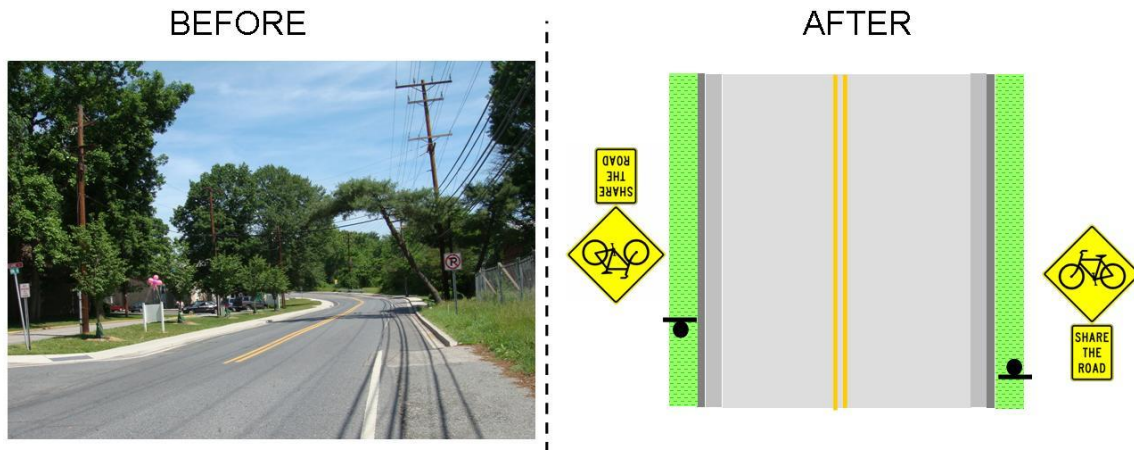
Figure 26: Before and After Signage/Striping Improvements for Bowie Rd.
