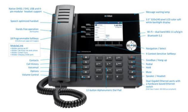
The 6920w is designed for power users who require a phone with a modern design that is flexible and delivers a high-quality communications experience. It provides flexible network connectivity options including wired Ethernet and built-in Wi-Fi to facilitate installation in work-at-home and corporate environments.
