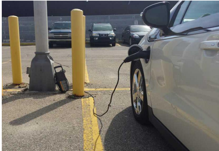
Photo 5. GM installs Level 1 outlets on parking lot lamp posts for convenient workplace charging.
