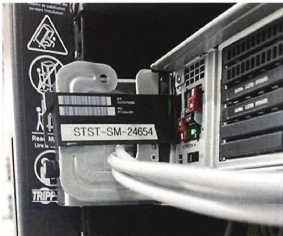
Figure 22. Large Tesla System Controller (1459155) Information Pull Tab Label (Example)
