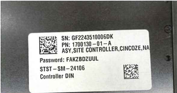
Figure 21. Large Tesla System Controller (1700130) Label on Side (Example)
