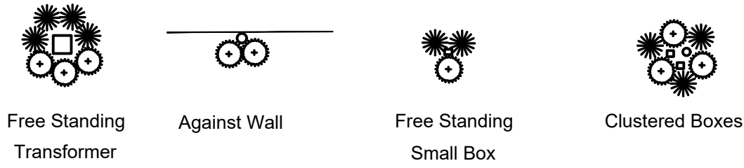
TYPICAL UTILITY BOX SCREENING DETAILS - NTS
