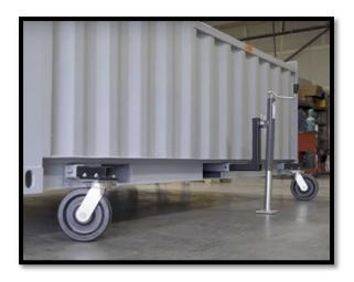
Casters and jack: Each Taylor'd Prop includes four high-quality shop-grade casters and a manual jack as standard features. The manual jack can be inserted into the front or back side to elevate the prop, allowing the casters to easily lock into place. This setup enables one or two trainees to move the prop effortlessly on hard surfaces. Each caster is equipped with a swivel lock to assist in maneuvering the prop.
