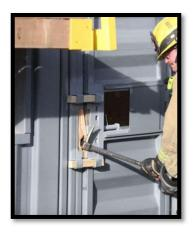
Force Doors: The setup includes two steel doors, one swinging outwards and the other inwards. These doors are equipped with a standard 2 in. x 6 in. wooden piece featuring two 1 in. holes and small sections of 2 in. x 4 in. wood. This design allows trainees to practice prying techniques with tools like the Halligan while maintaining door integrity. The wooden sections can be easily replaced after
