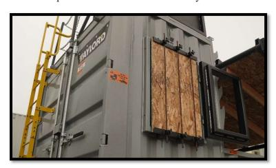
incorporates holes for screwing boards into place for transportation or sealing the setup. Additionally, the window includes a Denver Drill insert mounted on hinges, limiting the window's dimensions to 20 in. wide x 28 in. tall for Denver Drill practice. It also features a slot for sliding a 1.5 in. x 1.5 in. piece of wood on the container's interior to replicate a window sash.
