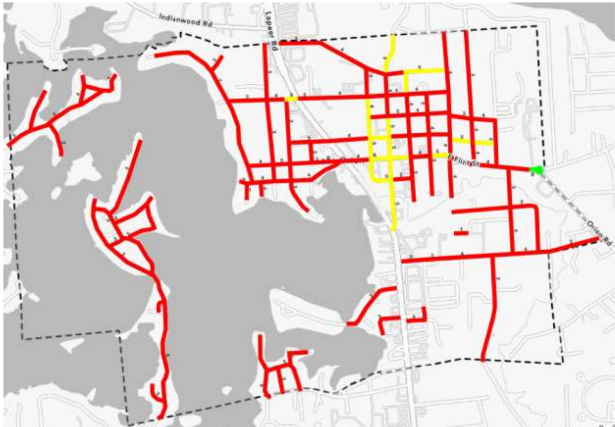
Figure 7: Map of the 2024 paved road condition in Good (PASER 10, 9, 8) shown in green, Fair (PASER 7, 6, 5) shown in yellow, and Poor (PASER 4, 3, 2, 1) shown in red. Only Roads owned by VLO are shown.
