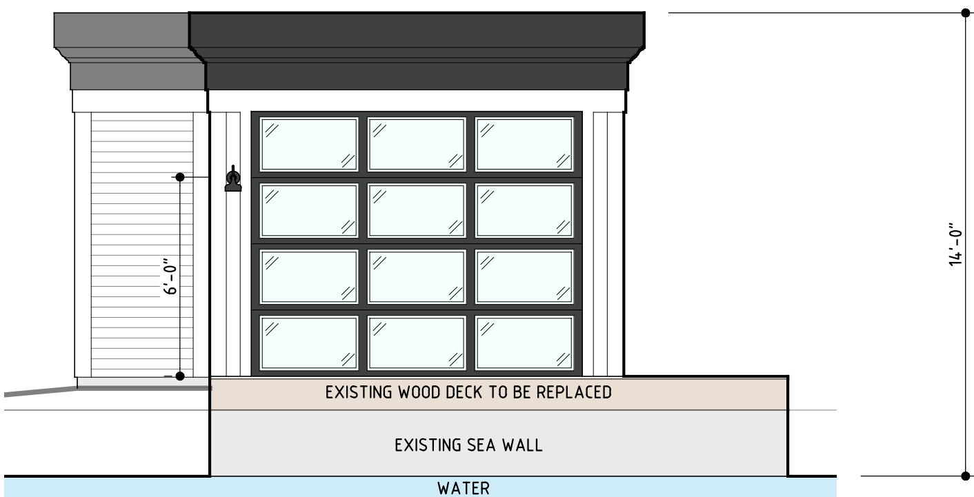
6 WEST ELEVATION SCALE: 1/4" = 1'
