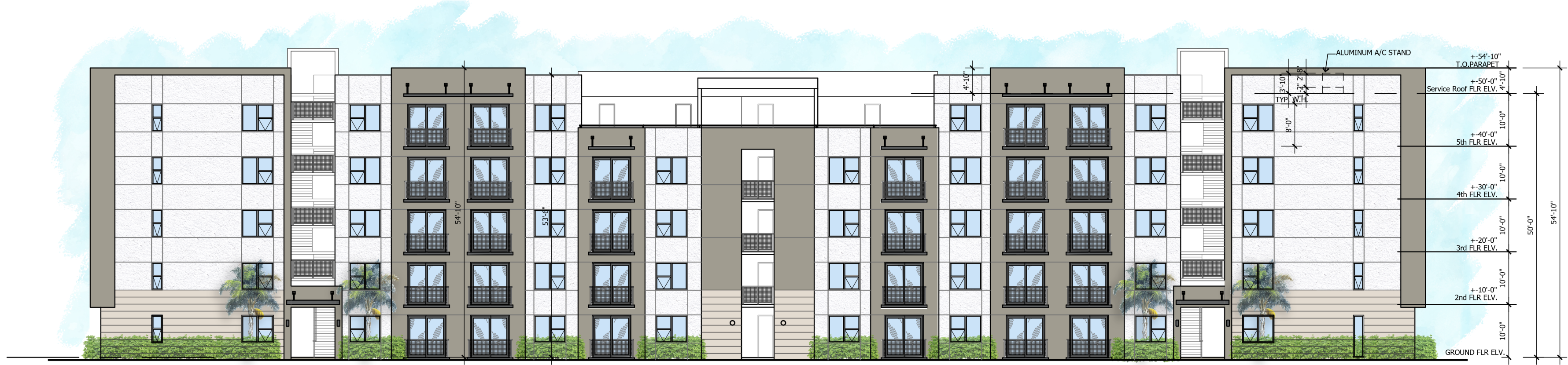
2 EAST ELEVATION LWS ELEVATIONS SCALE: 3/32"=1'-0"
