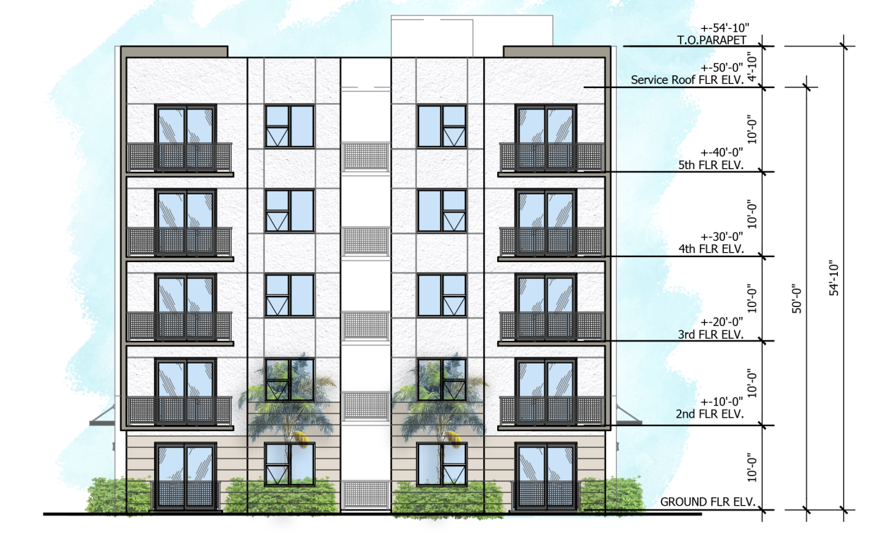
3 SOUTH ELEVATION LWS ELEVATIONS SCALE: 3/32"=1'-0"
