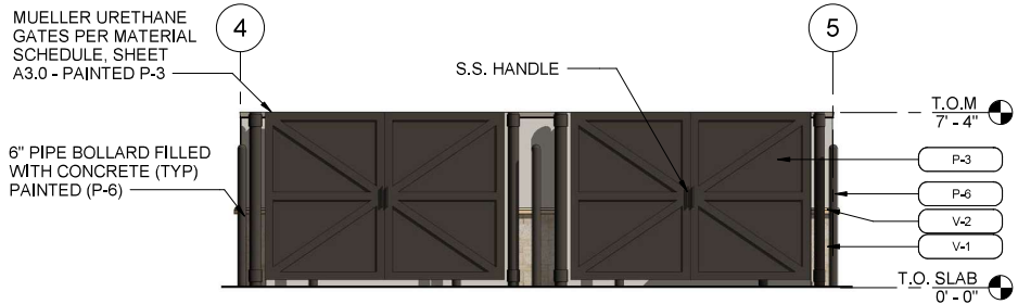
3 DUMPSTER FRONT ELEVATION SCALE: 1/4" = 1'-0"
