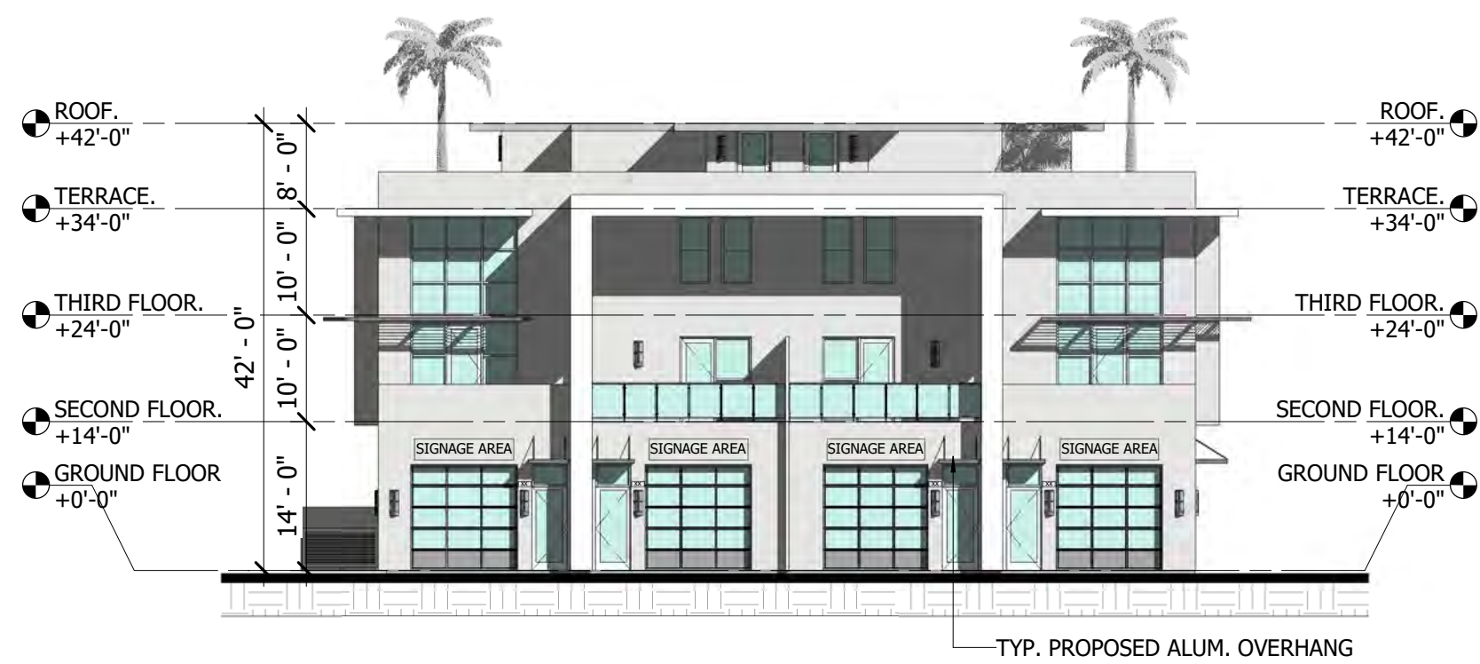
4 BLDG 1&3 - ELEVATION FACING INTERIOR PLAZA SCALE : 1/16" = 1'-0"
