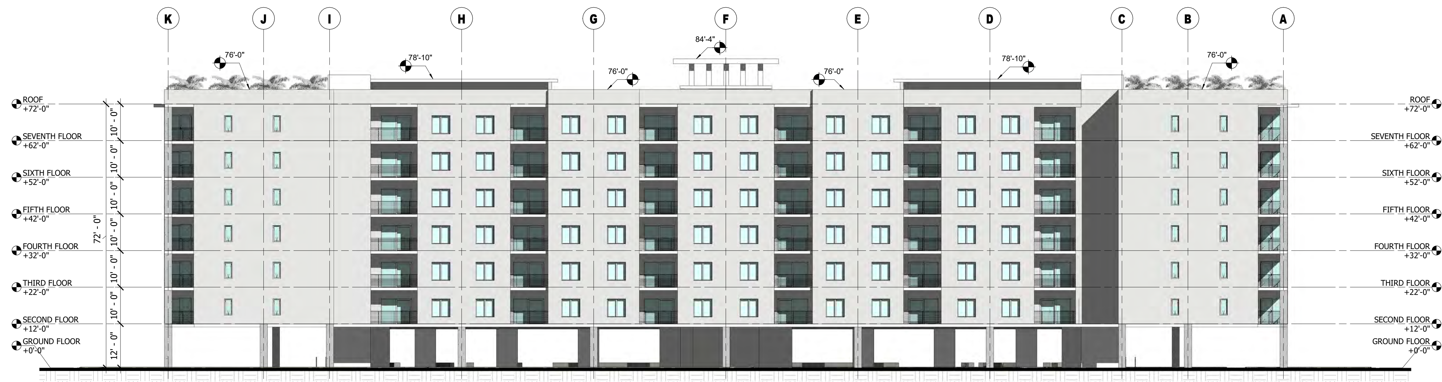
2 BLDG 2 - WEST ELEVATION SCALE : 1/16" = 1'-0"
