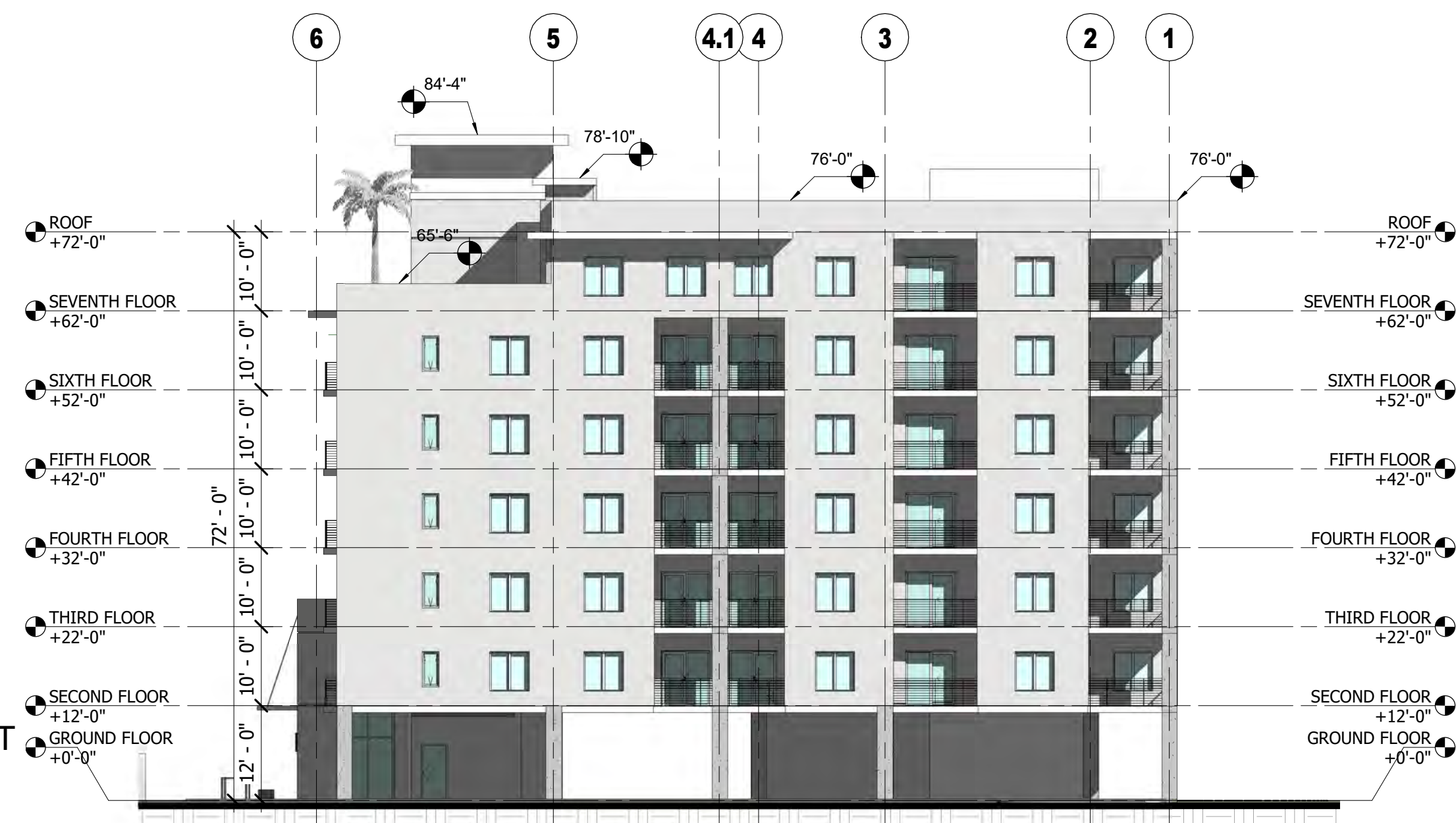
3 BLDG 2 - NORTH ELEVATION SCALE : 1/16" = 1'-0"
