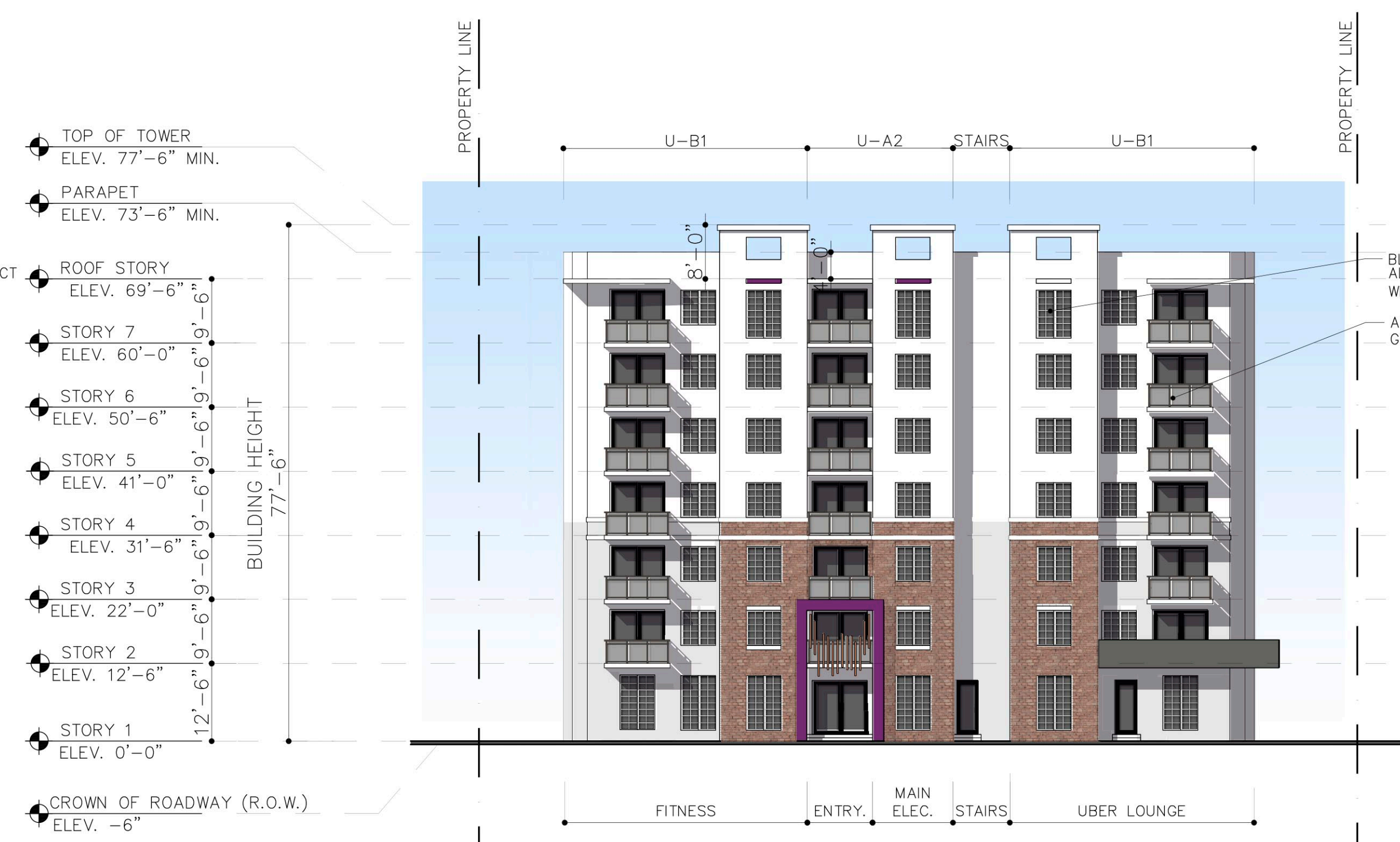
4 SOUTH BUILDING ELEVATION
