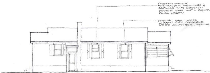
Existing Window and Door Replacement North Elevation
