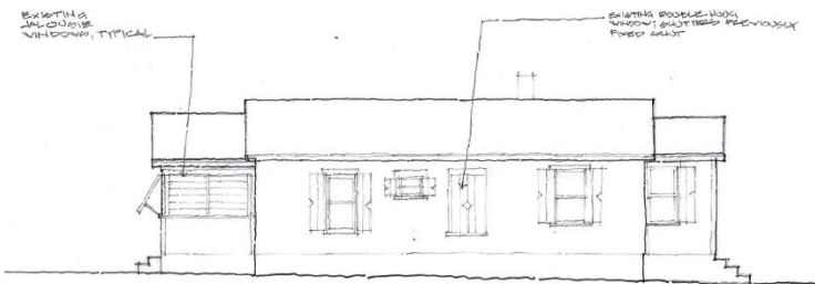
Existing Window and Door Replacement South Elevation
