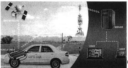
tracking and fleet management systems use a GPS transmitter/receiver and a small antenna on each vehicle that links it to the GPS network which can then monitor each vehicle's activity 24 X 7 X 365. The vehicle data is then downloaded into the user's master database, providing a permanent history of the entire fleet operation.
