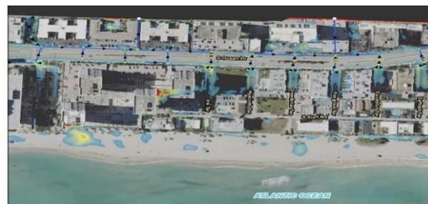
storm events with rainfall volumes of 1.57, 2.50, 2.70, 3.08 and 3.6 inches per hour, respectively. Results indicated that the Built scenario will not eliminate all flooding from minor rainfall storm events. The results indicated that for the larger (major) 3 and 5-year/24-hour design storm events, the Built Scenario is successful in decreasing the depth (4-6") and duration of flooding.
