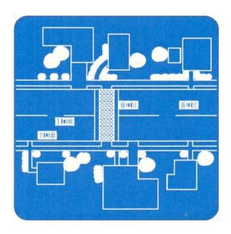
Raised crosswalks are speed tables outfitted with crosswalk markings and signage to channel pedestrian crossings. They provide pedestrians with a level street crossing, and by increasing the level of the crossing, pedestrians are more visible to approaching motorists.
