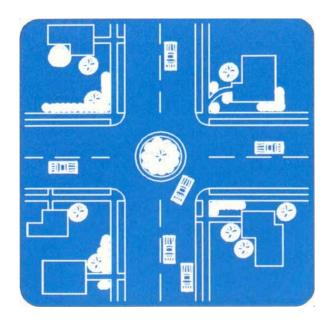
Traffic circles are raised islands placed in intersections around which traffic circulates. They are not intended for high-volume or large vehicle traffic. Traffic circles sometimes employ stop or signal control or give priority to entering vehicles. Some traffic circles impose control measures within the circulating roadway or are designed with weaving areas to resolve conflicting movements.
