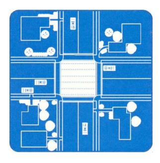
Raised intersections are flat raised areas (3 to 4 inches) that cover an entire intersection with ramps on all approaches and often with brick or other textured materials on the flat section. By modifying the level of the intersection, crosswalks are more readily perceived by motorists to be "pedestrian territory". The objectives are to slow traffic and reduce the number and severity of crashes.
