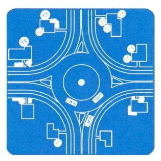
A raised circular structure that deflects the flow of traffic in a counter-clockwise direction around the circle. The objectives of roundabouts are to slow traffic and reduce the number and severity of crashes. Roundabouts are designed to accommodate all sizes of vehicles. Unlike traffic circles, roundabouts are used on higher-volume streets.
