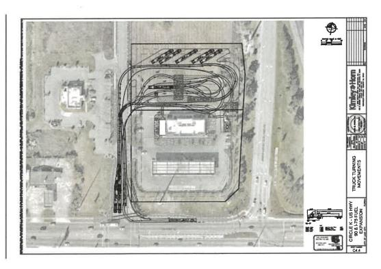
Below is a second drawing of the Truck Turning Movements, which depicts tractor trailer rig access to the high flow diesel pump service bays and alternative egress by exiting through the existing Circle K parking lot and automobile service station area.
