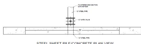
STEEL SHEET PILE/CONCRETE PLAN VIEW
