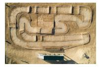
Remote control vehicles range in size from 17 to 22 inches long and 8 to 15 inches wide. These vehicles run on dirt and paved tracks with 6 to 10 wide lanes. The overall size of the track can be any size based on budget. Typically, the track will be approximately 60 x 120 feet in size with an elevated stand for the controllers to better view the track and operate the vehicles. Larger tracks have been constructed
