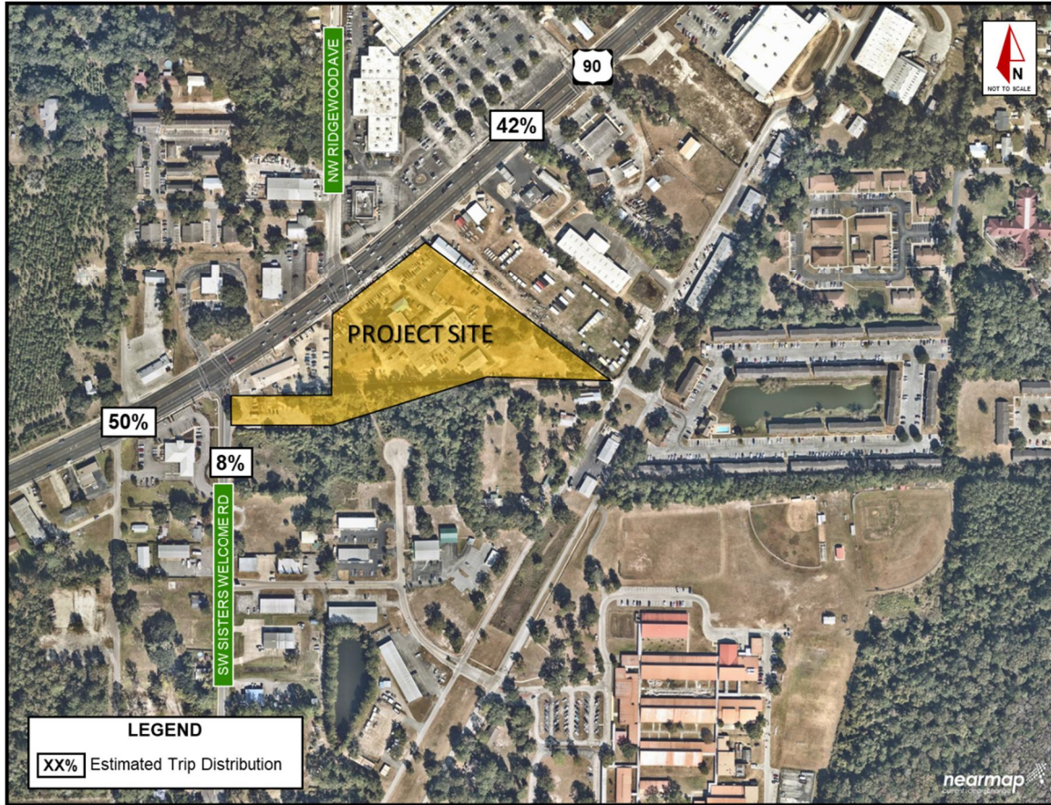
Figure 2: Approximate Trip Distribution
