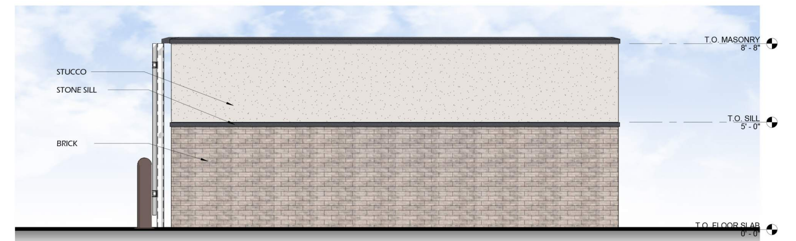
⑤ SIDE ELEVATION 2 - TRASH COMPOUND 3/8" = 1'-0"
