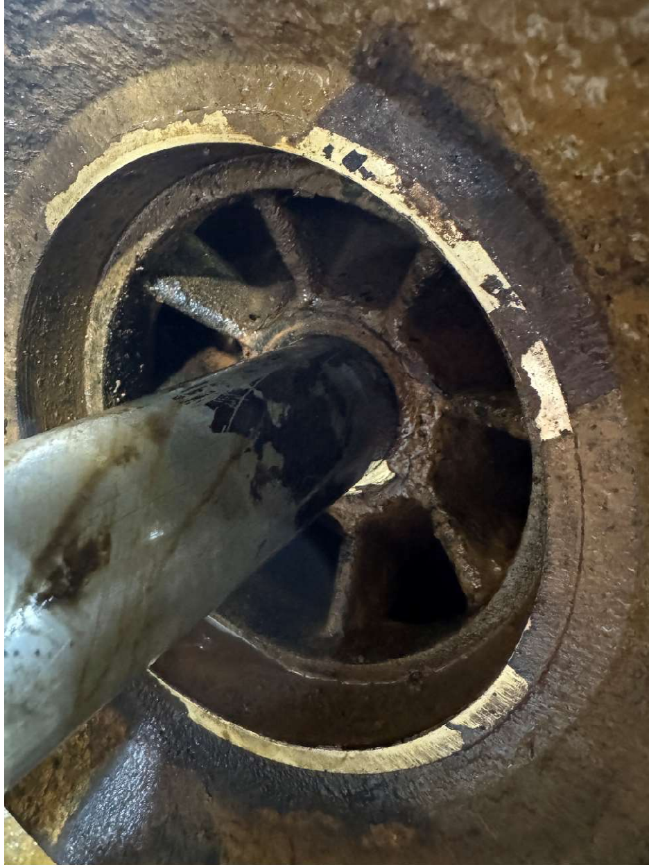
Top Side of Intermediate Pump Casting that was stuck on the pump shaft due to build up and sediment.
