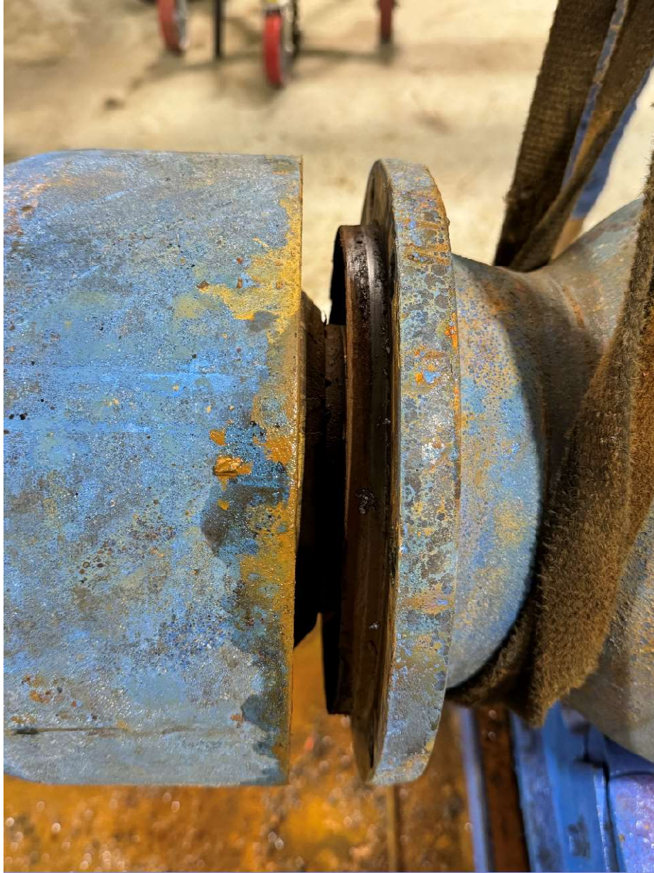
Side View Close up of intermediate and impeller stuck on shaft as pictured previously.
