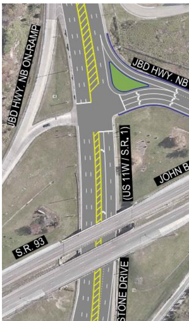
Figure 5. Proposed NB Off-Ramp Geometry for Improvement A
