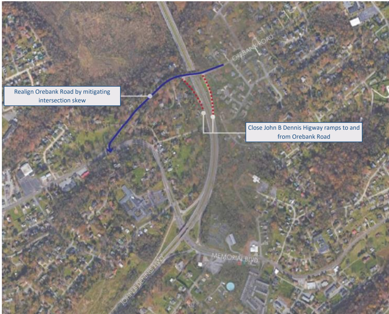
Figure 5-6 Orebank Road Interchange Closure
