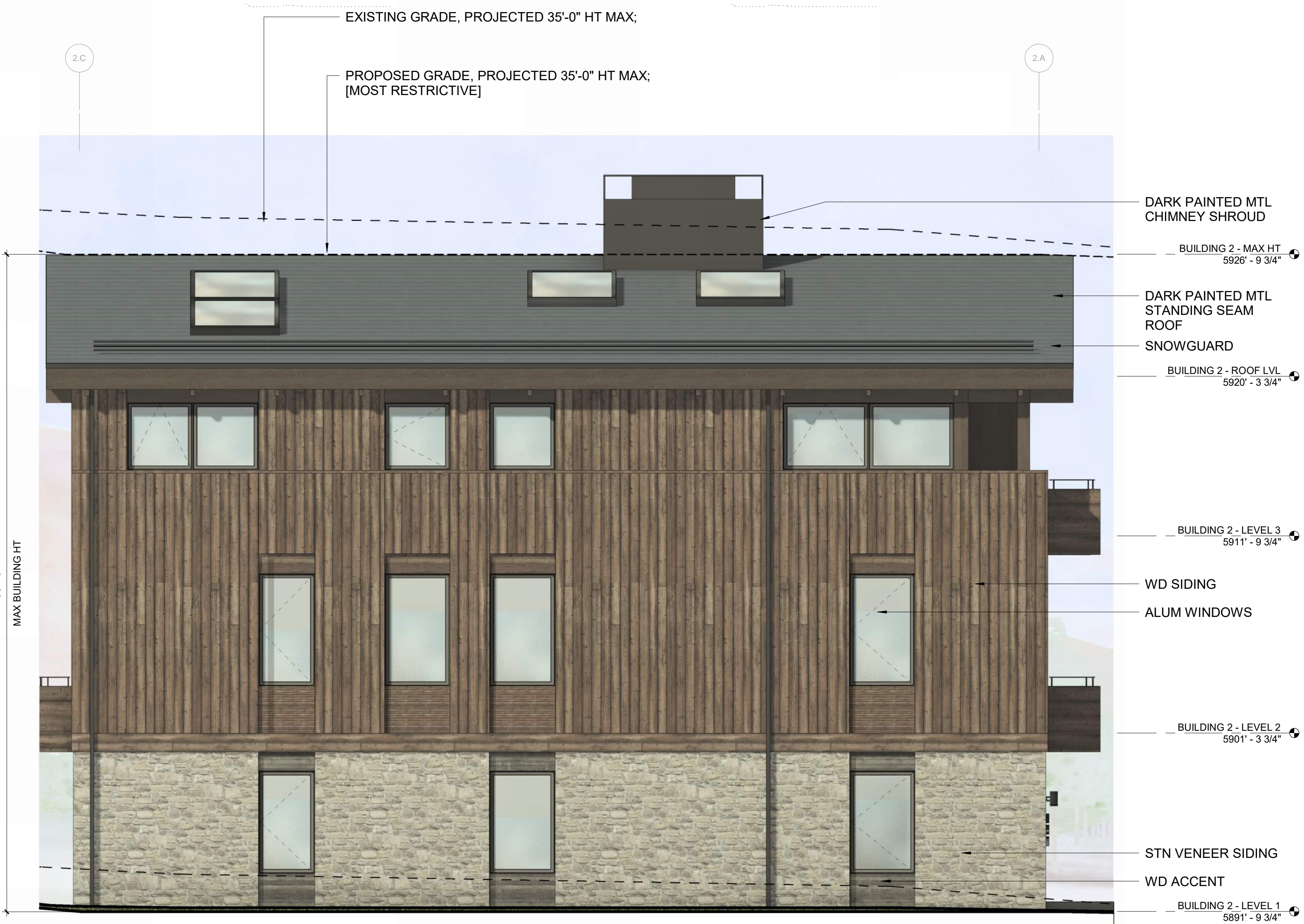
2 1/4" = 1'-0" BUILDING 2 / ELEVATION - EAST
