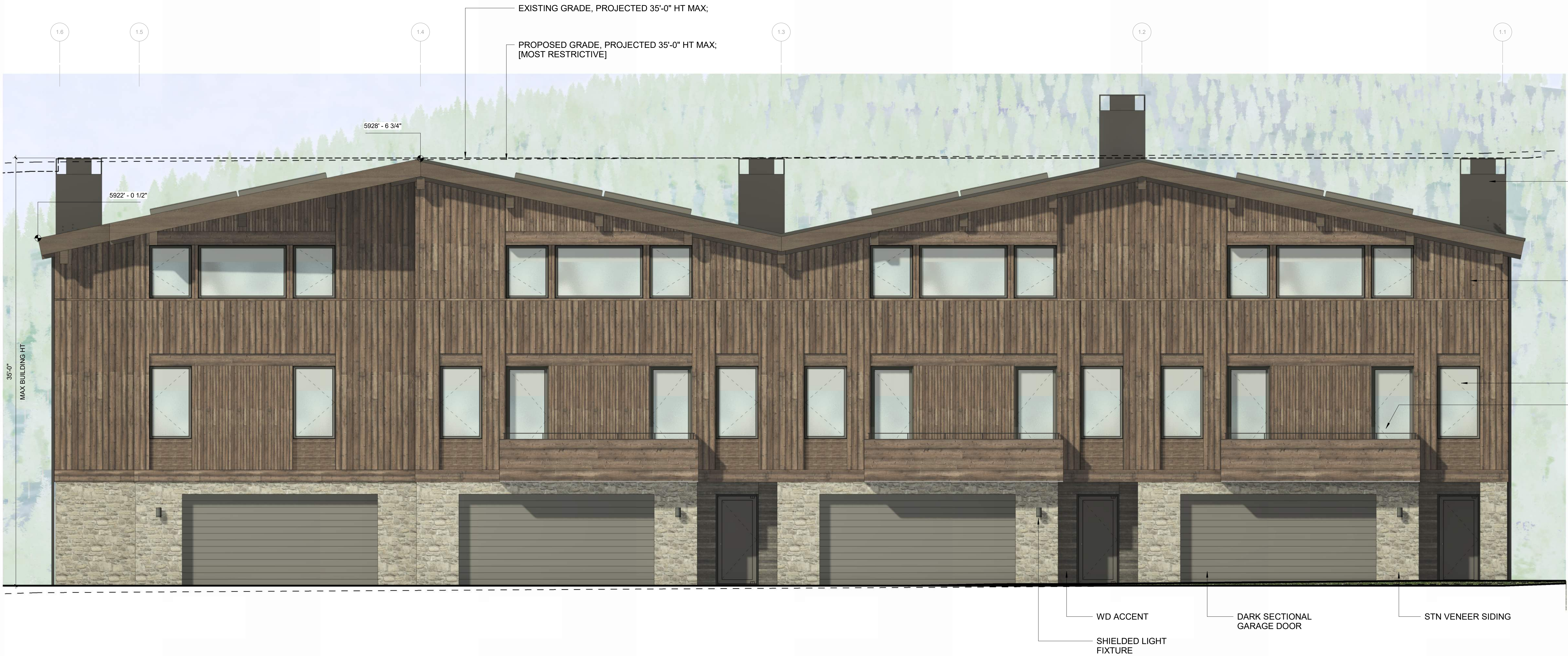
2 1/4" = 1'-0" BUILDING 1 / ELEVATION - WEST
