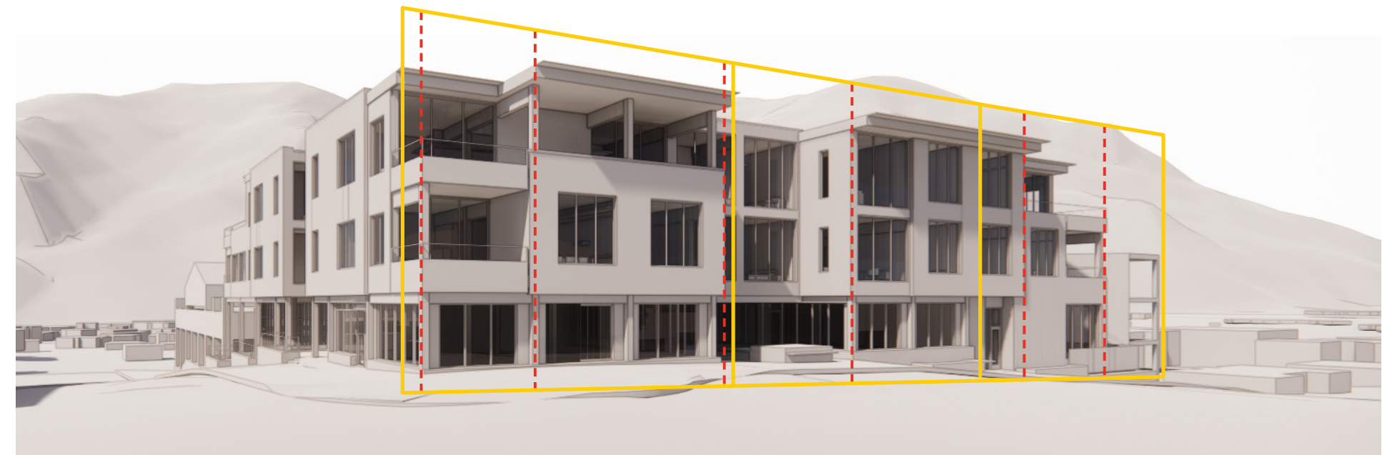
STRUCTURE: CLT grid module informs plan organization.
