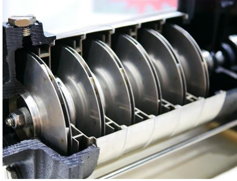
Figure 4. Typical Centrifugal Blower Cross-Section
