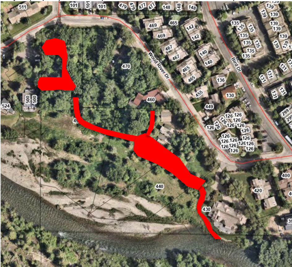
Figure 1 Aerial image of approximate drainage channels and ponds
