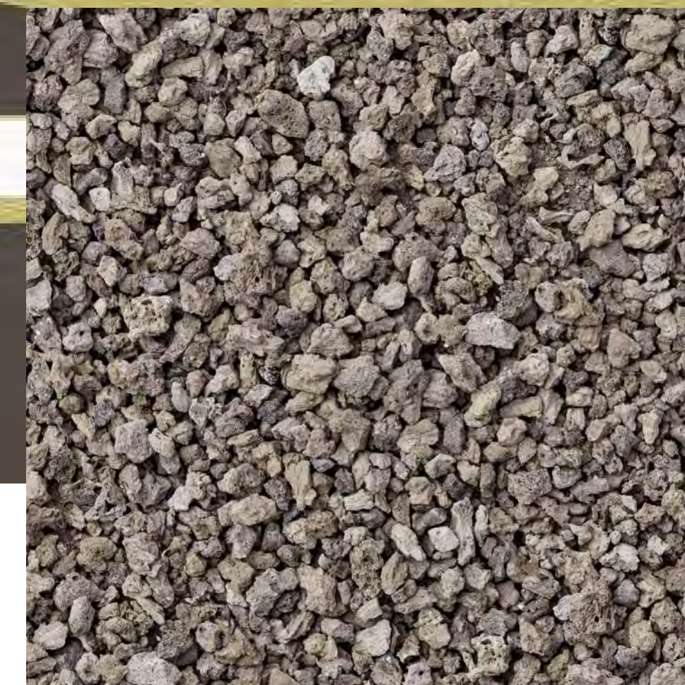
GRAVEL BALLAST OVER MEMBRANE: 3/4" SMOOTH GRAVEL
