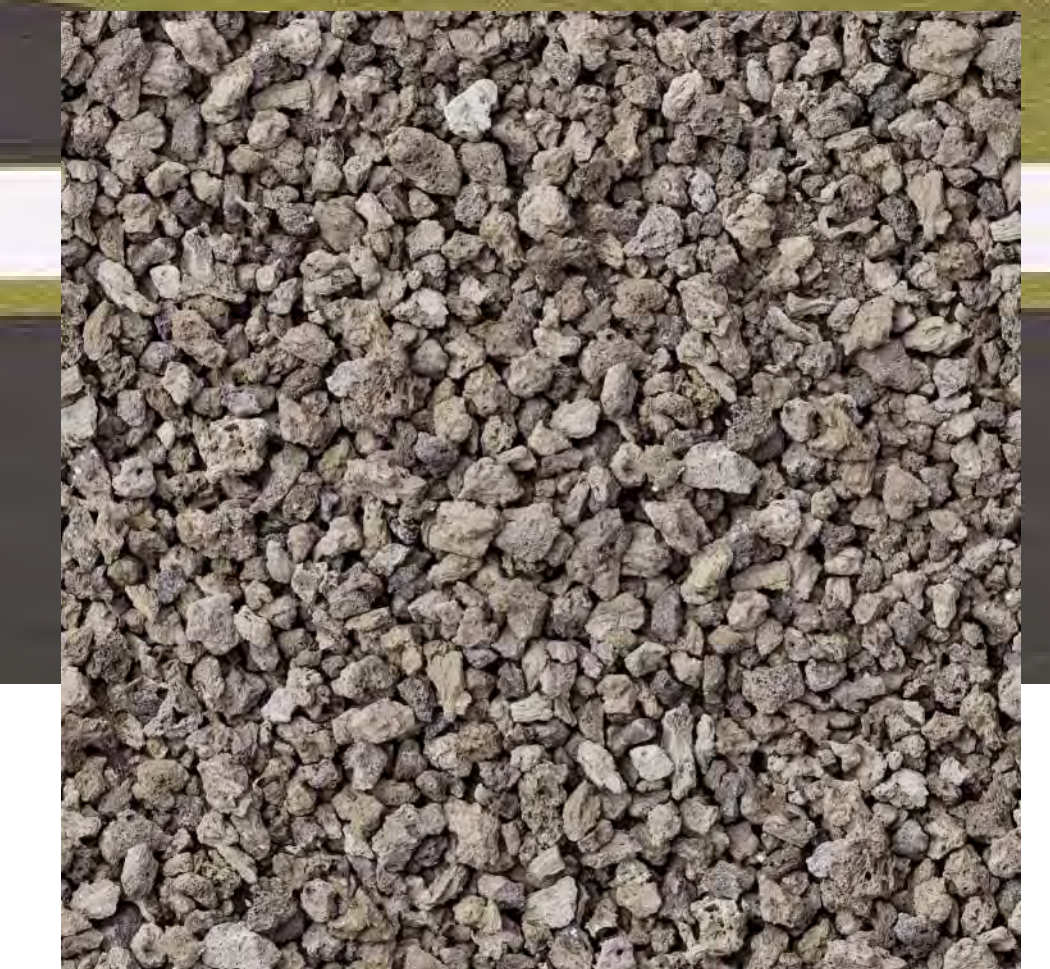
GRAVEL BALLAST OVER MEMBRANE: 3/4" SMOOTH GRAVEL
