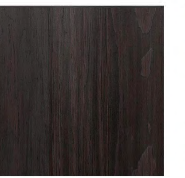
MAT 4 - Wood siding, Kebony, 1x6 vertical shiplap, color to be Hewn.com Krakatoa
