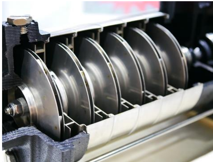
Figure 4-4. Typical centrifugal blower cross-section
