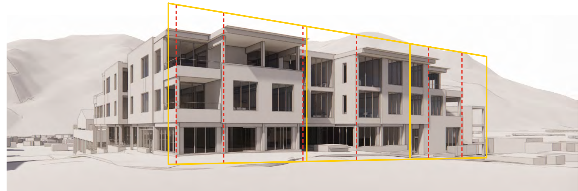
STRUCTURE: CLT grid module informs plan organization.
