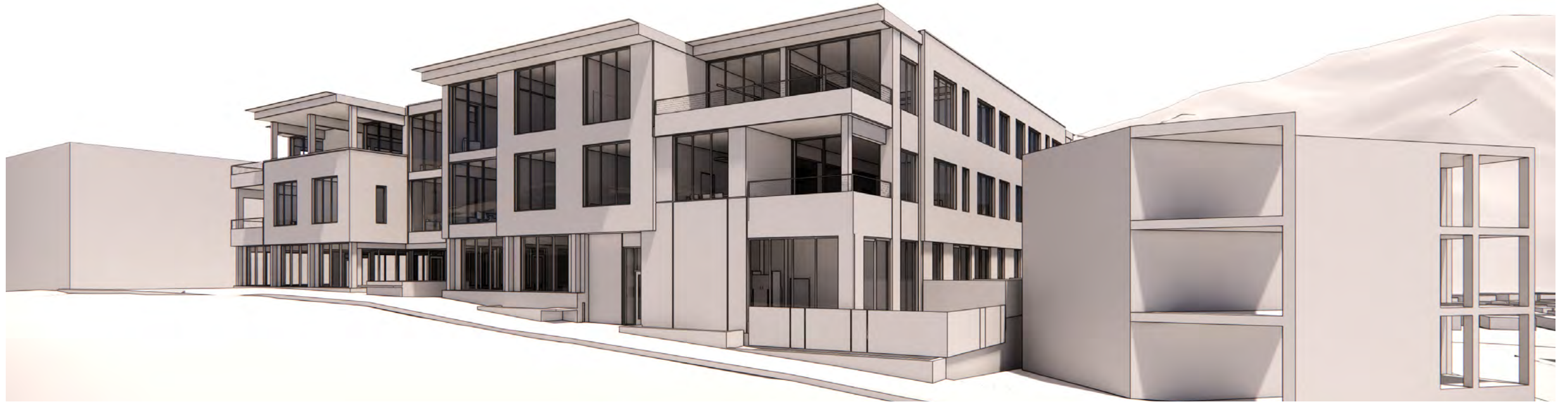
NEW PROPOSED ROOF OVERHANGS ALONG 1ST AVE
