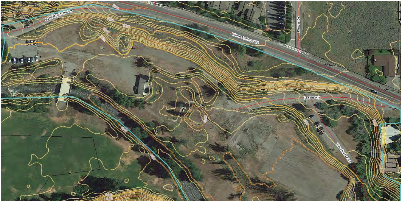
Figure 1: Existing Road Alignments and Grades
