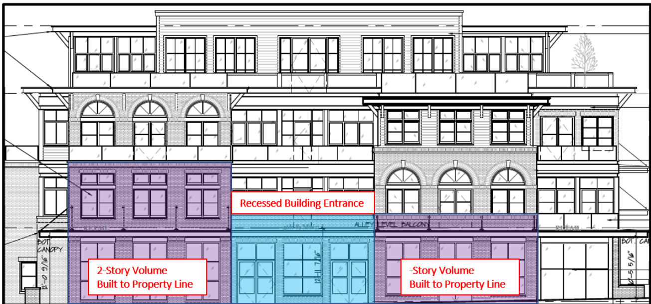
Figure 4: Main Street Building-Mass Modulation
