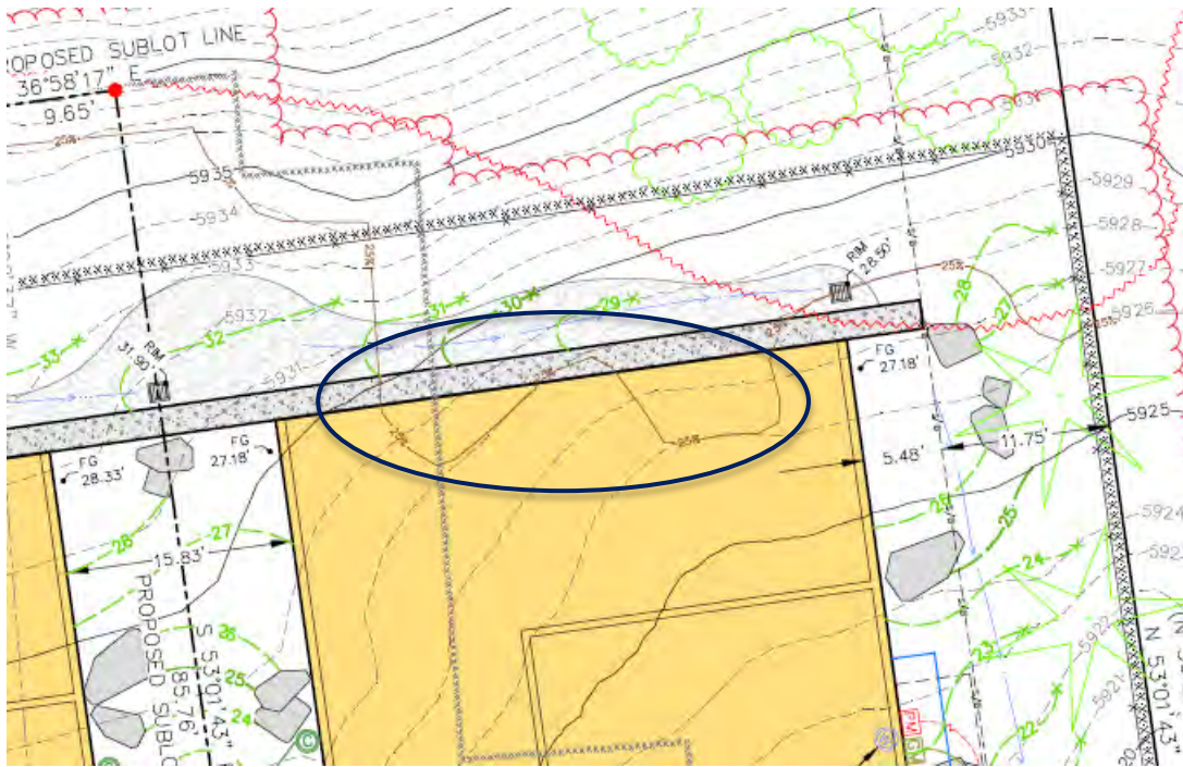
Figure 3. Encroachment of building into 25% slope (circled in black).
