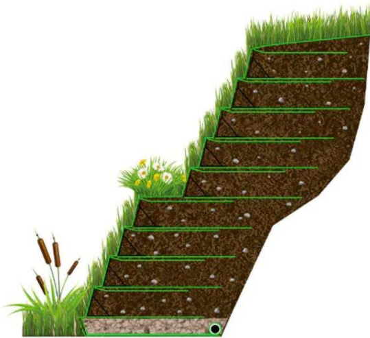
Figure 8 - Wrapped-Face Geosynthetic Reinforced Slope
