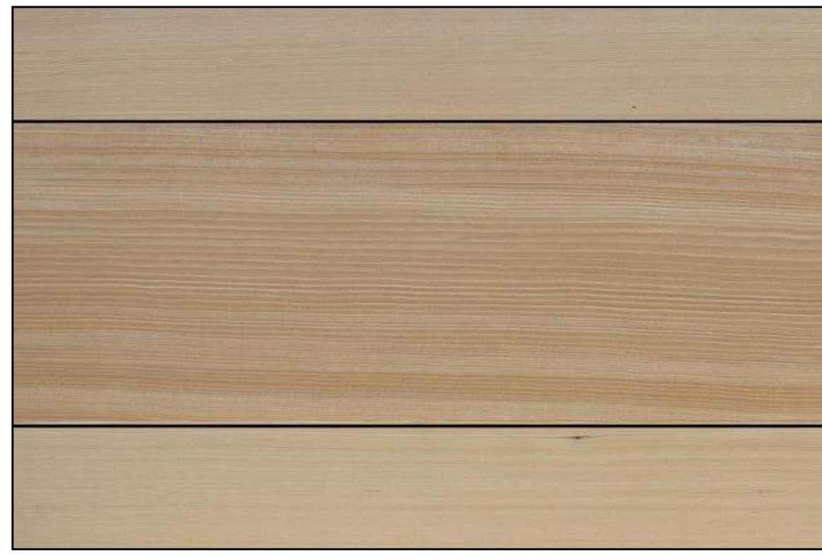
EXTERIOR FINISH 5 (EF-5): EXTERIOR WOOD SOFFIT. RESAWN TIMBER CO. VERTICAL GRAIN WESTERN HEMLOCK
