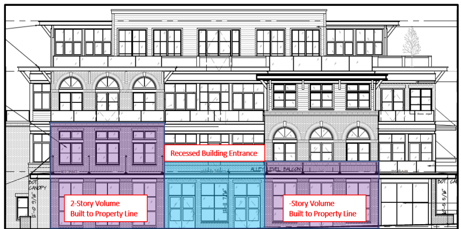
Figure 2: Main Street Building-Mass Modulation
