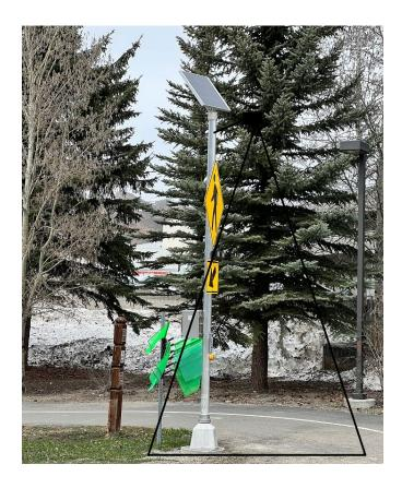
A little hard to draw in a 2d drawing the area of focus, but hopefully those pictures give you some idea. The sensor has a 95 degree field of view, so very wide angle view.
