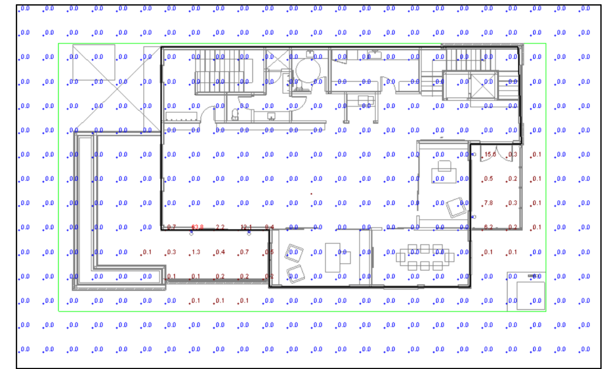
SITE LIGHTING PHOTOMETRICS - SECOND FLOOR BY: HELIUS LIGHTING NOT TO SCALE
