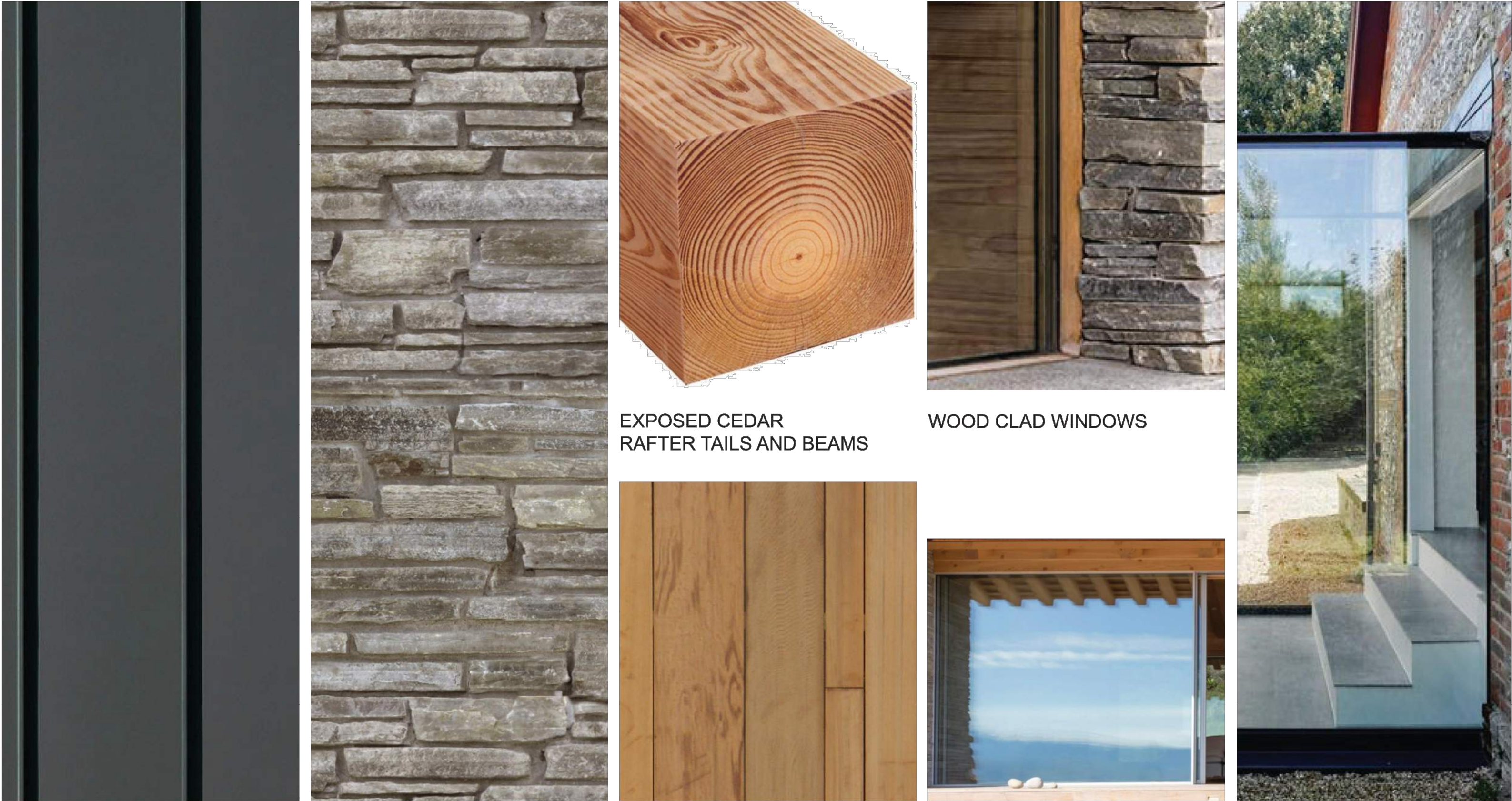
CHARCOAL STANDING SEAM METAL ROOF OAKLEY STONE VENEER NATURAL FINISH CEDAR VERTICAL PLANKING AND SOFFITS STEEL LIFT AND SLIDE GLASS DOORS TRANSPARENT GLASS CONNECTORS
