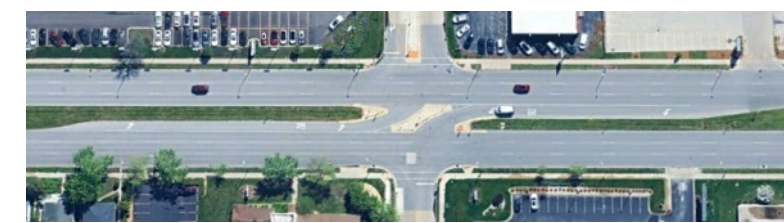
Left-in/Right-in/Right-out Access Example
