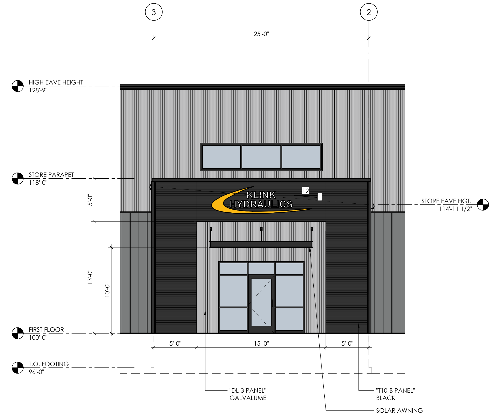
3 SOUTH ELEVATION - HYD. STORE ENTRY 3/16" = 1'-0"
