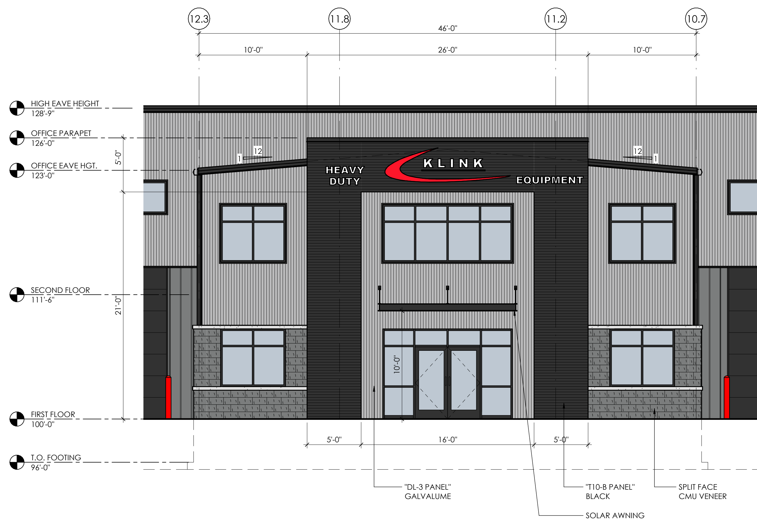
4 SOUTH ELEVATION - OFFICE ENTRY 3/16" = 1'-0"
