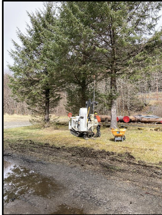
Photo 6: Looking north at soil boring SB12 being advanced north of the paved driveway. SB12 was subsequently converted into monitoring well MW2, the up-gradient sentinel well.
