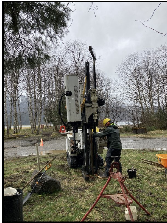
Photo 1: Looking south at soil boring SB01 being advanced next to the 2019 G.E.C. water sampling point TH3 (white pipe sticking up from ground left of the drill rig). SB01 was subsequently converted into monitoring well MW1.
