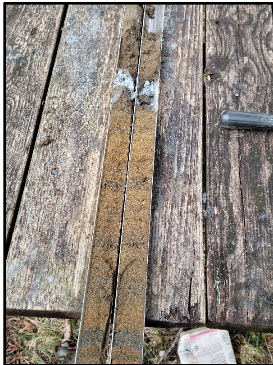
Photo 4: Looking down at the opened soil core retrieved from boring SB02 (0 to 5 feet). Note the coarse sandy tailing soil material.
