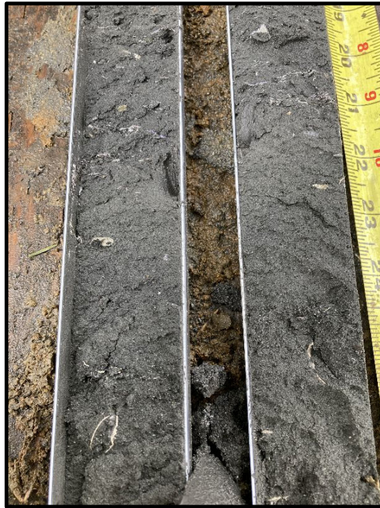
Photo 7: Looking down at a soil core retrieved from boring SB12 (5 to 10 feet). Note the very fine sandy silt with shell fragments is a native marine sediment which directly underlies the sandy tailings soil material.
