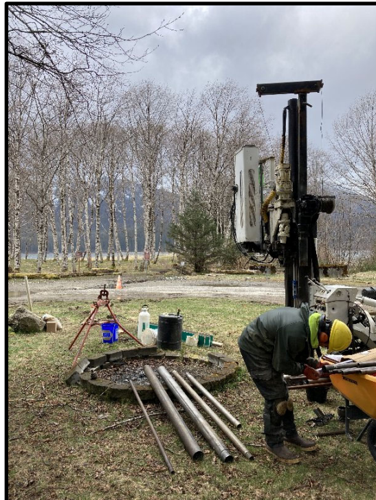
Photo 2: Looking south at soil boring SB02 being advanced next to the fire pit.
