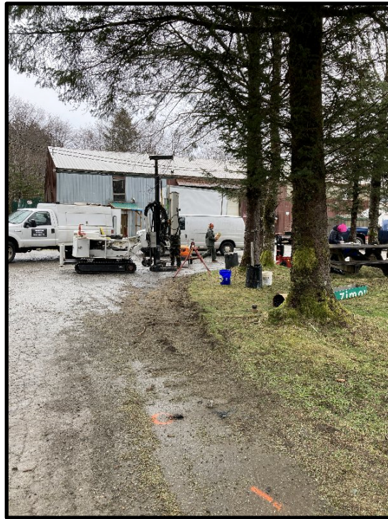
Photo 5: Looking east at soil boring SB07 being advanced. Note the hole for boring SB06 is visible in the foreground.
