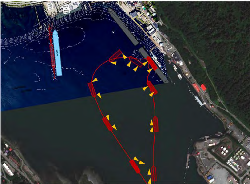
Figure (26). Maneuvers of Coast Guard 420-foot Coast Guard icebreaker HEALY to and from the Port of Juneau dock with two tugs assisting, with proposed HTD overlaid.
