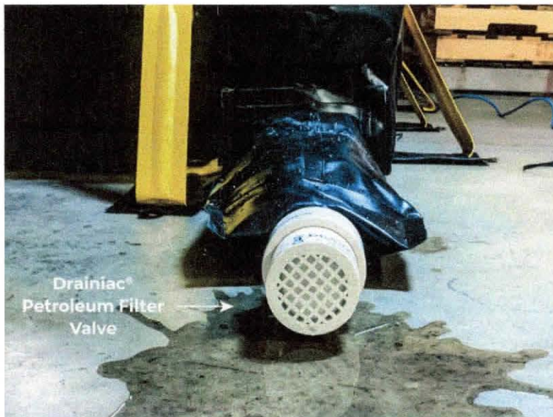
Drainiac® Petroleum Filter Valve attaches to the Snoutlet Drain, filters sheen from rain water and automatically shuts off during a spill.
