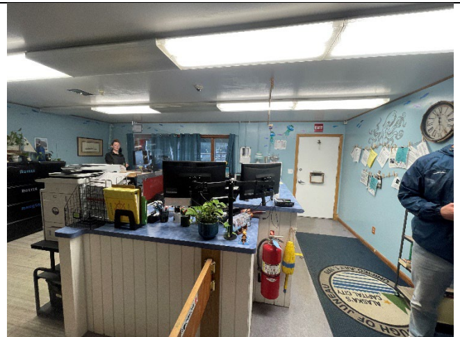
Aurora Harbor Office: Front main office area accessibility requirements should be evaluated further. Exit signage is not illuminated.
