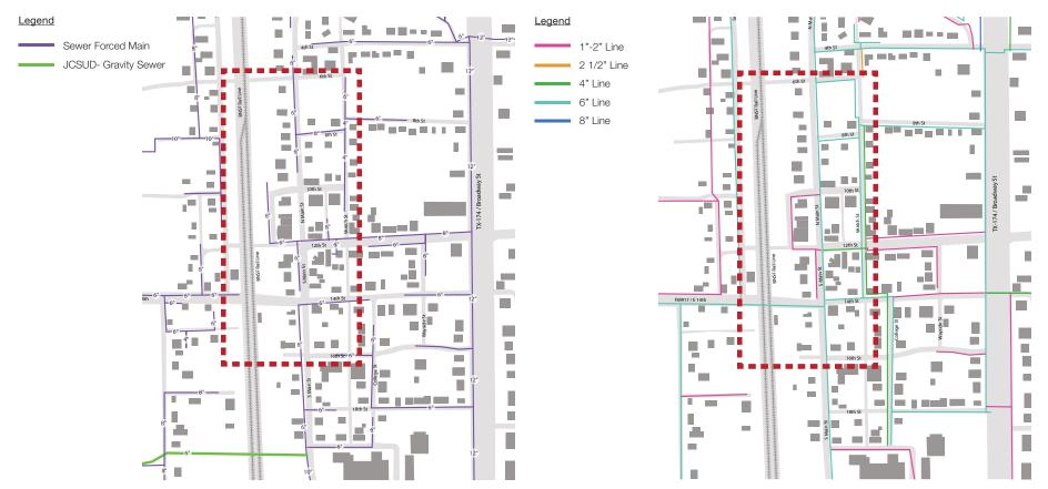
Figure 19: Existing Sewer Infrastructure Diagram
